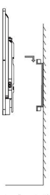
Figure 3-5 Wall Mounting Side View
