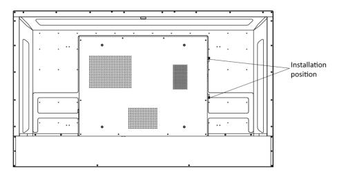
**Figure 3-3 Internal Computer Installation**
