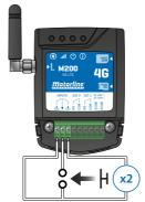
4 • Give two pulses simultaneously on the two inputs IN1 IN2 and GND;
