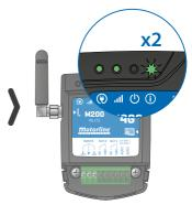
6 · Wait until the ACT LED starts flashing 2 times with 1 second interval;
