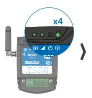
3 · Wait until the ACT LED starts flashing 4 times with 1 second interval;
