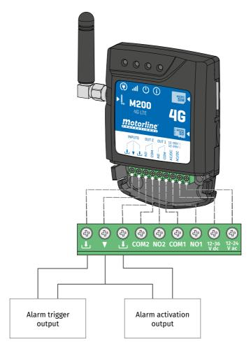
As soon as the alarm is triggered, Input 2 is activated and the system starts making calls to the contact list in order of listing until a contact answers.
