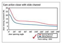
dormakaba's unique cam action closer combined with a slide arm and channel do not experience an increase in the opening resistance but a rapid fall in
