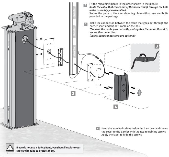
C • Tighten the two screws to secure.
