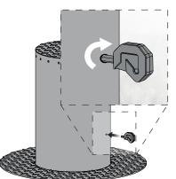
To unlock the electromechanical pillar, insert the key into the slot and turn in a clockwise direction.
