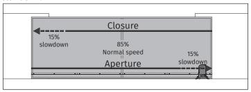
The control board automatically sets a slowdown in opening and closing equal to 15% of the total course.
