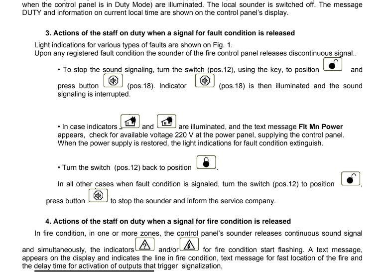
Duty Mode is the status where no fire condition or fault condition is detected in the fire alarm system.
